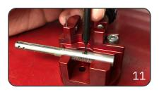
Step 11: Place the tool body on the front bed of the mounting fixture and insert the split pin with the assembly tool and a small hammer.
