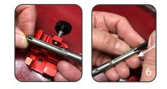
Step 6: Push the spring back - at the front edge of the spring - over the pre-loaded split pin by using the pin of the mounting fixture first and then the assembly tool pin.
