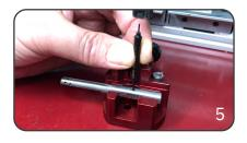
Step 5: Remove the split pin by inserting the assembly tool and drive it slowly out of the tool body with a small hammer.
