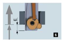
In back working feed the backward deburring is executed until position E. Then exit in rapid traverse.
