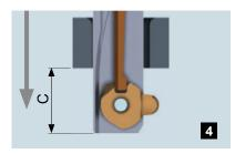
In order to make the blade snap out again, the tool has to be positioned beyond the rear bore edge by measurement C.
