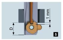
Travel the tool back in rapid feed below the rear material surface of the hole or the burr **D**.
