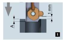
Rapid traverse of the cutting unit of the tool above the top material surface of hole or burr. Referencing the front edge of the cutting blade A.
