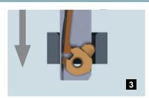
Rapid traverse through the hole. The surface of the hole cannot be damaged.
